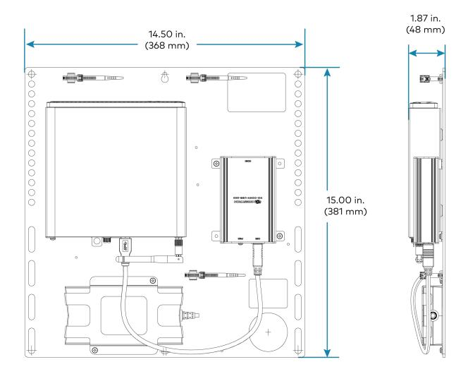
UC Bracket Assembly with HD-CONV-USB-200
