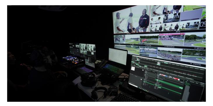
Sponsor logos and brand bugs also play out of the TriCaster's internal DDR into the alpha channel. The TriCaster, Titler Broadcast and Resolume systems are connected via the NDI 5 Profile of a Netgear M2450 series AV Line Switch.
