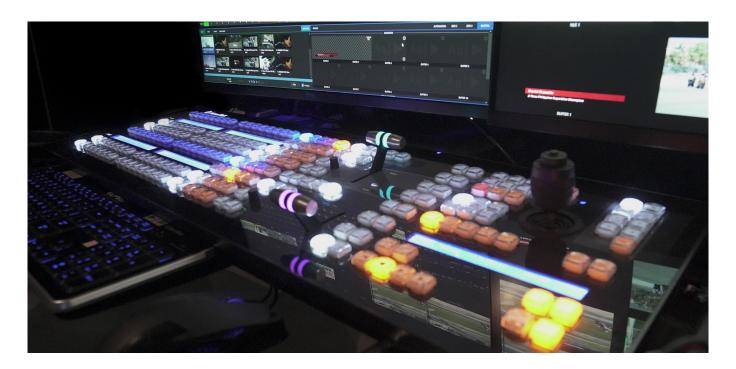
A critical element of the production was the use of NDI to transfer high-resolution video sources, such as full-screen racing statistics and lower-third graphics, in real-time from a Resolume Arena Media Server and NewBlue Titler Broadcast into TriCaster's NDI -ready alpha channel inputs for keying.
